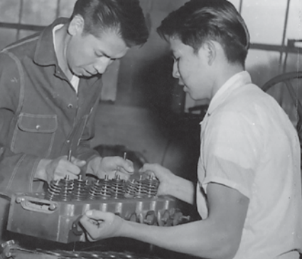
Auto mechanic trainees overhaul a car by replacing the head, ca. 1955. FCC-OHS
